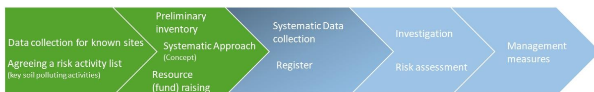
Fig. 2: Stepwise approach: from potential contaminating activities over a systematic methodology to a register and management measures
